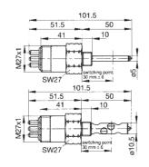
Capacitive level sensors designed to monitor either water or oils and fuel. Normally closed output switches when uncovered by medium. Connection to switch is made by bayonet connector, please order separately.
