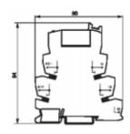
A space saving package comprising relay, and IP20 DIN rail mounting base measuring only 6.2mm wide. Relays and sockets can also be purchased separately. Base fitted with LED indicator and back emf protection (diode dc version). Note 230V ac version uses 60V dc relay, socket has integral diode bridge,
